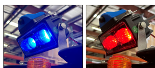
Turns from solid BLUE to flashing Red when a pedestrian is detected.
