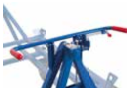
Release the basic position by pressing down the handle
