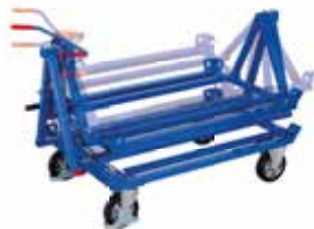
The desired tilt position can be reached by swivelling the tipping unit and locked by releasing the handle
