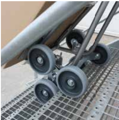
Aluminium stair-climber truck | with 2 three-arm star wheels
