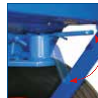
Automatic securing of the drawbar eye
