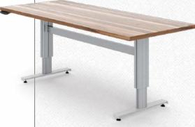
The base frame **SM-4** consists of four lifting columns arranged in a rectangle and connected by crossbars. The lifting columns are equipped with a foot plate including adjustable rubber feet. The table top is attached directly to the adapter plates of the lifting column **SM.**
