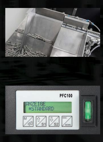
The feed material is quietly fed in stages over linear feed plates from the storage container towards the feed rails.
