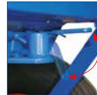
Automatic securing of the drawbar eye
